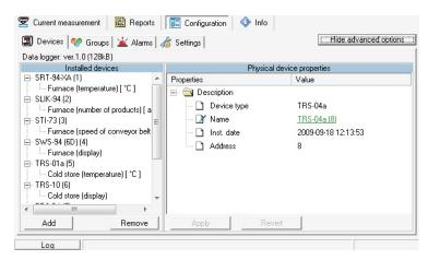
SimCorder is designed for acquisition, archiving, visualization and reporting of measurement data from SIMEX products equipped with RS-485 serial communication interface with Modbus RTU protocol. Converters like RS-485/USB or RS-485/RS-232 allow connecting multiple devices to a computer via USB or
