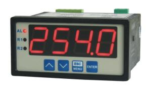
The PAC-94T temperature meter has one input: thermoresistance (Pt100/500/1000) or thermocouple (K, S, J, T, N, R, B, E). Measurement is linearised by the polynomial characteristics. The device with thermocouple input has additional measurement range (-10 ÷ 90 mV) mainly for diagnostics of measurement circuits. A 4-digits, 20-millimetre LED display enables seeing of measured values from a distance. The RS-485 enables data transmission in production process monitoring systems
