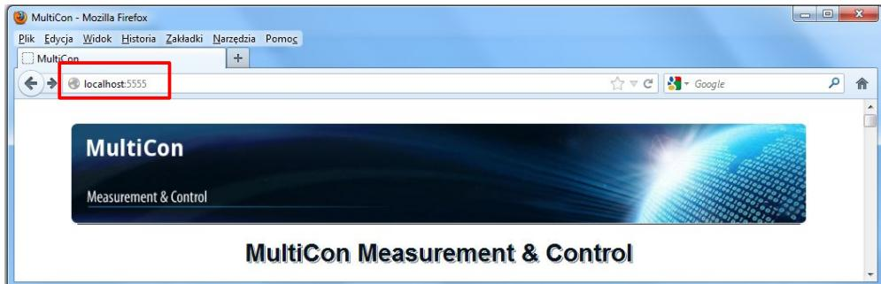
*Fig. 1. Web address settings for the 'MultiCon Emulator' in web browser.*
